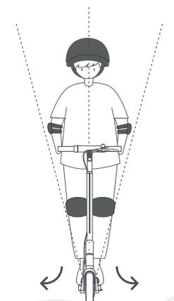
12.When you need to stop, release the acceleration handle to reduce speed, squeeze and brake the handlebar. Lay down the foot support and let the vehicle lean slightly in the foot support direction so that the foot support touches the ground, and the vehicle can be stabilized.
