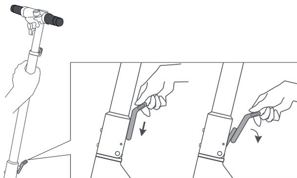
① Hold the front tube, press the folding handle down and then open it outwards;
