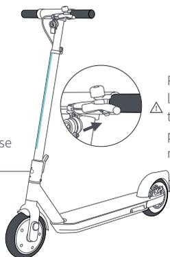
⚠ Press the brake lever to confirm that braking power is normal.
