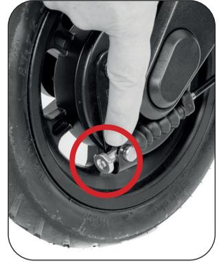
3. Now pull the brake cable along the recess on the brake lever until it fits into the guide at the end of the brake lever.
