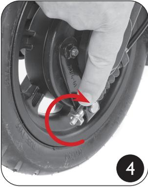
4. Now adjust the adjustment screw of the front brake so that no grinding noise can be heard when turning the wheel.
