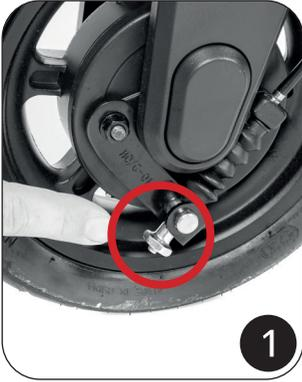
1. After you have mounted the handlebar, first turn the front brake adjustment screw counterclockwise until it is flush with the thread.
