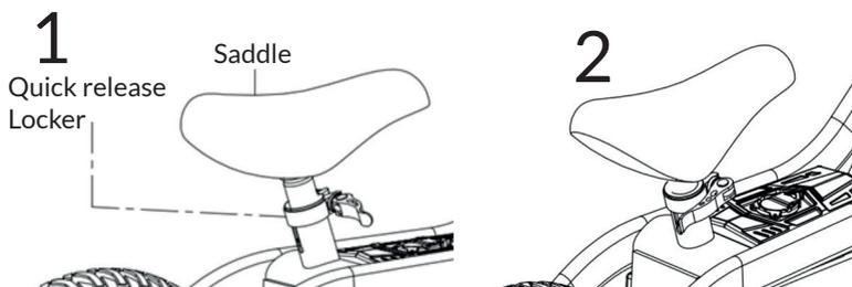
1. Loosen the lock and place the saddle in the correct position.
